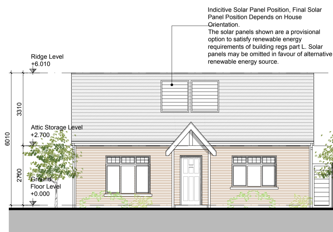
FRONT ELEVATION - House Type H2
