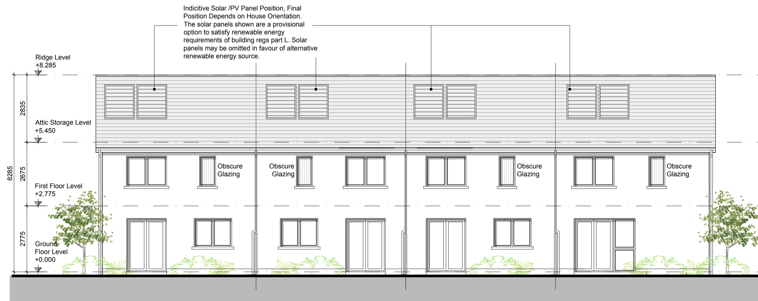
REAR ELEVATION (NORTH) - House Types F1-F-F-F2
