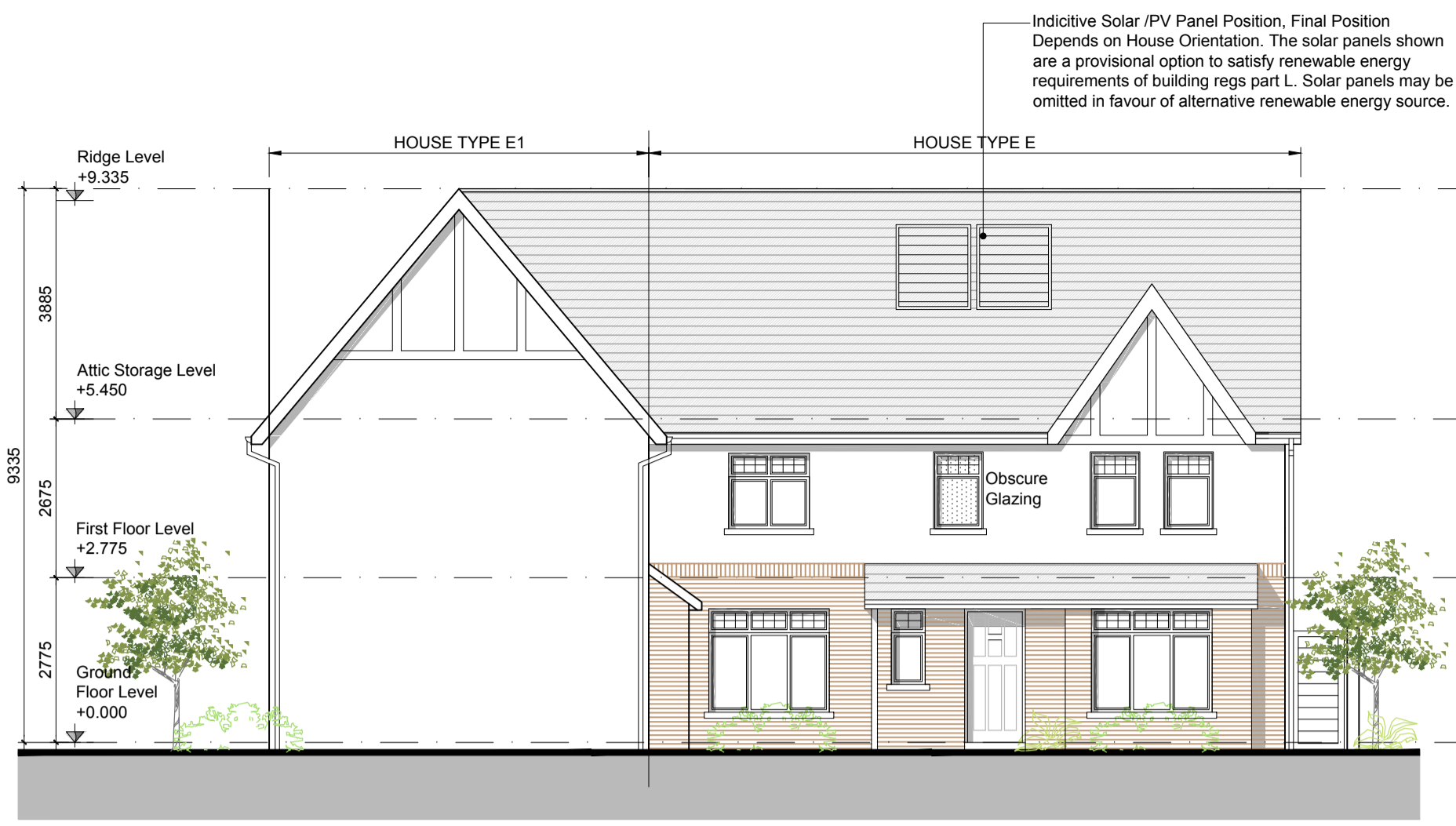
FRONT ELEVATION (EAST) - House Type E1-E
